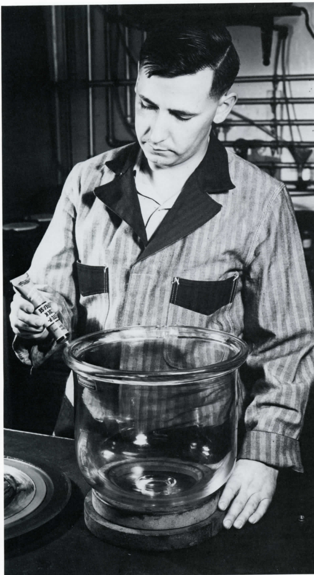
Dow Corning's first product was DC-4 Compound, a grease-like material that sealed aircraft ignitions, preventing arcing—a common problem in high-altitude flying. The end of World War II signaled the end of government contracts for this vital silicone compound.
