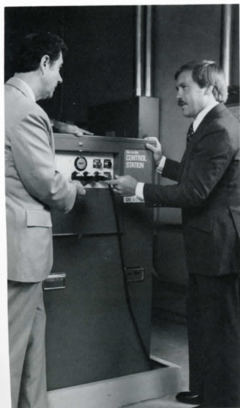
The RetroSil™ System, introduced in 1982, is a complete process to remove PCB fluids from electrical transformers. Doug Layne (left) and Bruce Shook look over a RetroSil System control station. (1982)
